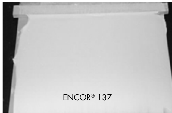
Figure 3. Fiber Tear testing illustrates the excellent durability of joint compounds based on ENCOR® 137 latex.
